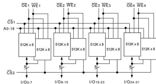
NOTE:  $\overline{CS}_1$  &  $\overline{CS}_2$  are used as bank select
