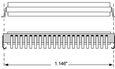
The WEDC 84 lead G3 CQFP fills the same fit and function as the JEDEC 84 lead CQFJ or 84 PLCC. But the G3 has the TCE and lead inspection advantage of the CQFP form.
